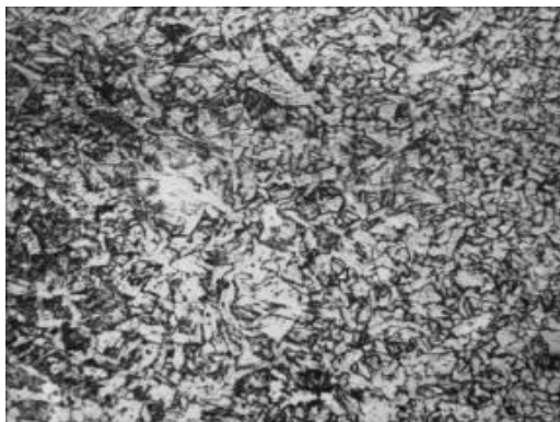
Fig 6 Location Weld/HAZ 100X
